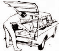
Tail door lifts up almost within overall length (a blessing in a tight spot). While it's up you can stand under it (see how the shape keeps off the rain).
